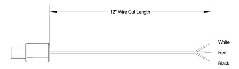
Specifications: Mounting: 1/2" NPT Housing: Nickel-Plated Prism: Fused Glass
