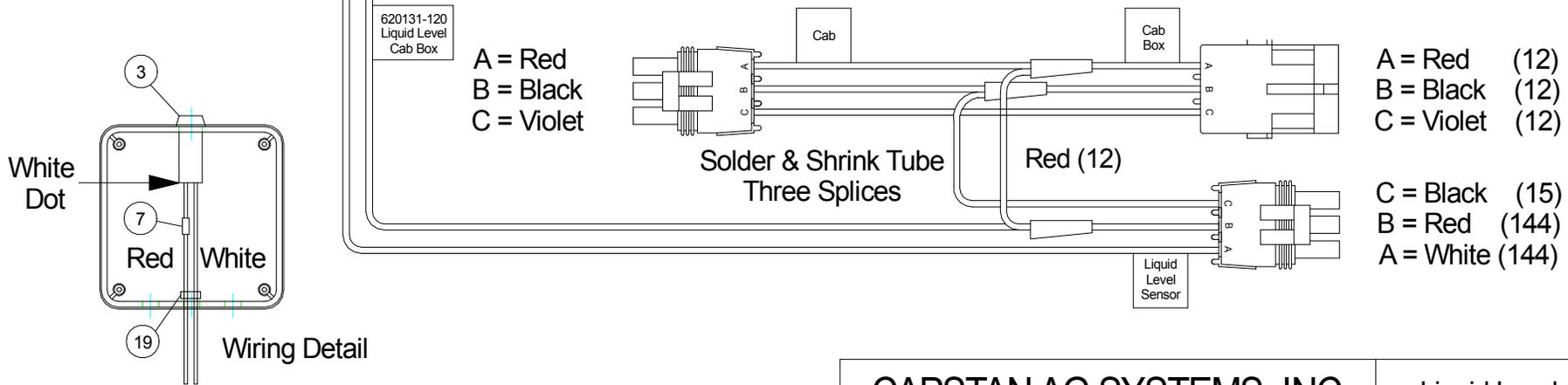
Note 1: Use Cable Tie, Around Harness, Inside Box, for Strain Relief.
