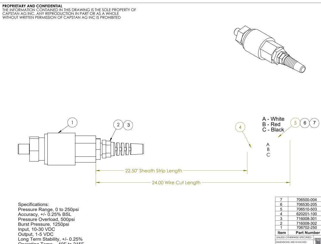
Long Term Stability, +/- 0.25% Operating Temp., -40F to 215F Compensated Range -4F to 185F Total Error Band EMI/RFI Protected, CE Mark UL Listed
