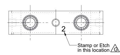
ø Tap Drill Into Passage Shown 1/4" FNPT Threads A/R Three Ports **⇒** 0.75"
