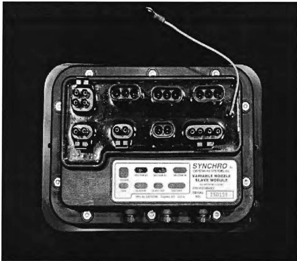
Figure 5. - Detailed connections and “pin-out” of the Synchro Slave Flow Control Module. This is the front view and the label is in the position we’ll call the “lower right” of the module.
