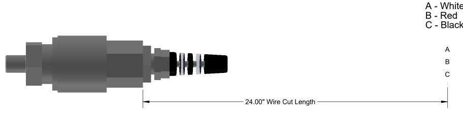
Specifications: Pressure Range, 0 to 100psi Accuracy, +/- 0.3% BSL Pressure Overload, 300psi Burst Pressure, 500psi Input, 10-30 VDC Output, 1-5 VDC Long Term Stability, +/- 0.25% Operating Temp., -40C to 85C Compensated Range -25C to 75C Total Error Band EMI/RFI Protected, CE Mark UL Listed
