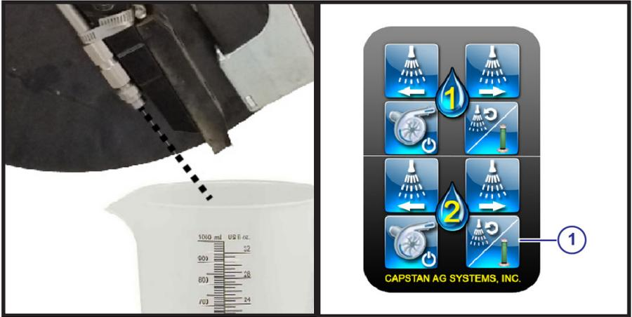
18. Put the calibration pitcher underneath the spray nozzle on row #1 of the planter.
