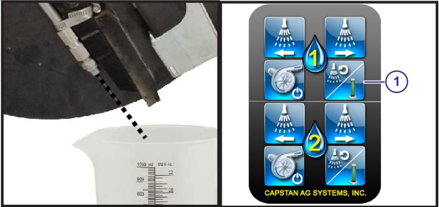
6. Put the calibration pitcher underneath the spray nozzle on row #1 of the planter.
