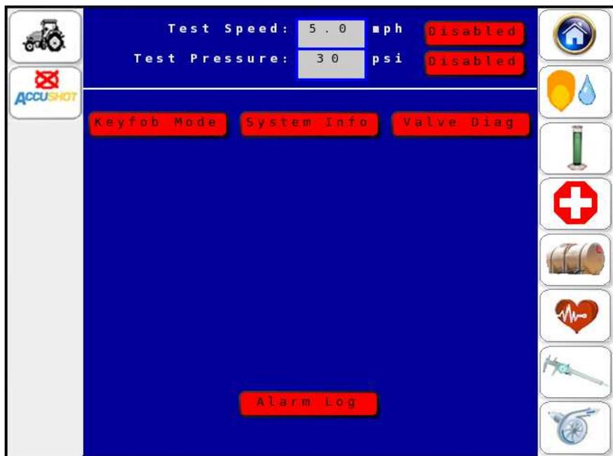
Select and toggle any of the red icons on the **DIAGNOSTIC** screen. The selected icon will turn green when activated. Make sure that the **MODE** icon on the **HOME** screen reads **OFF** to use the Key FOB and valve diagnostics.
