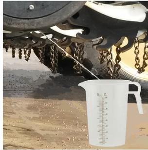
5. With the planter hydraulics engaged, touch the **START** icon on the **TIP CALIBRATION** Screen or press button (1) on the Key FOB to begin the tip calibration catch test.
