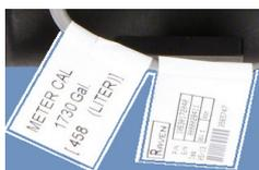
The Flowmeter Cal value entered must match the flowmeter (label) on the planter. The Flowmeter Cal Value IS NOT locked and must be set by the operator.
