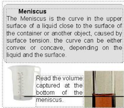
**NOTE:** Reading the calibration pitcher at or above the meniscus will cause an inaccurate GPA measurement.
